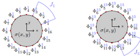
Figura 1: Given a domain with a conductivity distribution \sigma(x, y) , the EIT equipment is used to measure the electric potential \Phi_j^i at all the j \in [1, 16] electrodes for the current pattern injected into the pattern J_i .
